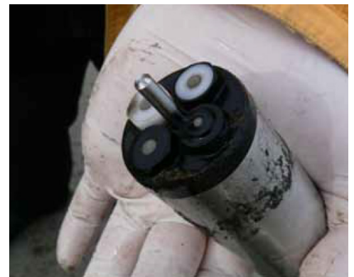
IQ Sensor Net System 2020 and VARiON® sensor in use at Glückstadt wastewater plant
